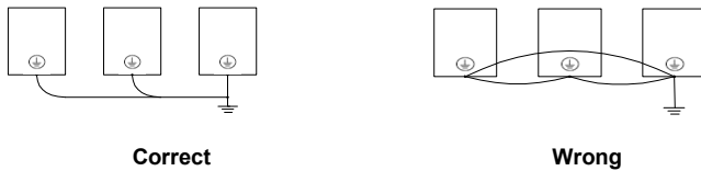
Fig. 3–3 Grounding wiring
