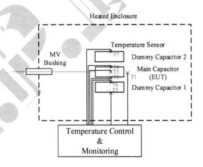
Figure 2: Sensors arrangement during the thermal stability test
