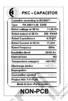
Figure 1: Nameplate of equipment under test
