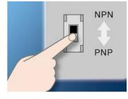
iE5 provides both PNP and NPN minor signal powers so that no matter what signal type the external controller adopts, +24V power can be applied.
