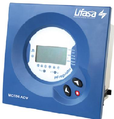
The power factor regulators, of types MCE06ADV and MCE12ADV measure the  $\cos\phi$  (sometimes called Displacement Power Factor, DPF) in a supply network and control the connection and disconnection of power capacitors in order to regulate such parameter.
