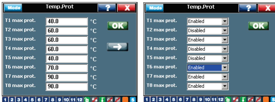
Figure 42: RVT temperature protection settings
