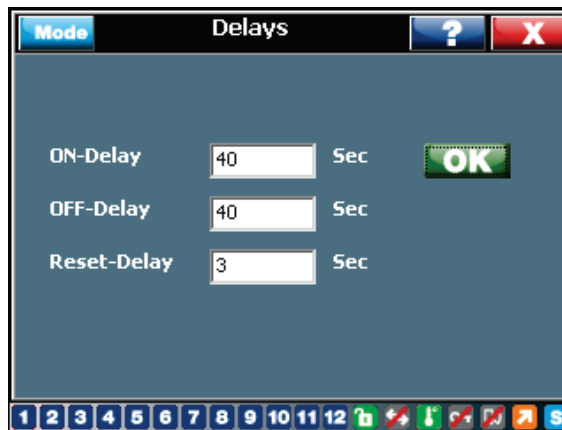
Figure 32: RVT delay settings
