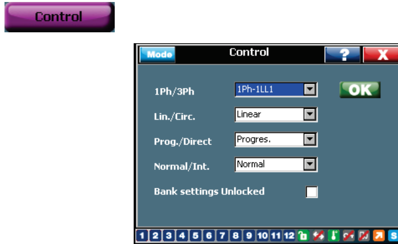
Figure 33: RVT bank control settings
