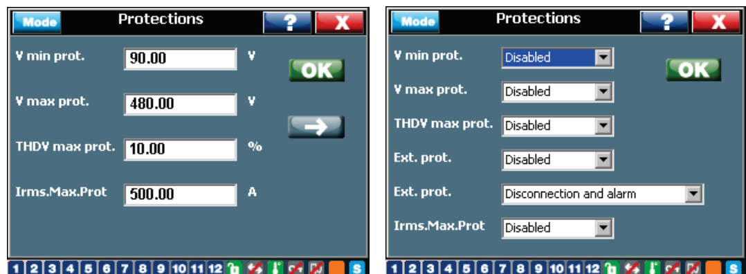
Figure 40: RVT protection settings
