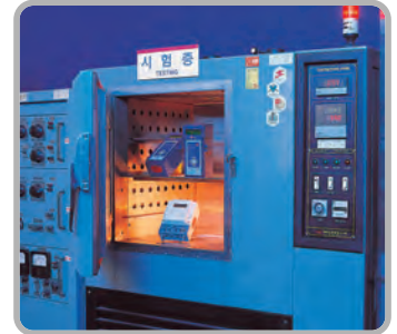
Environmental Test / Non-stop High Temperature Test
