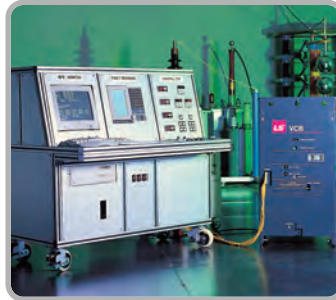
Characteristics Test / VCB Characteristics Test
