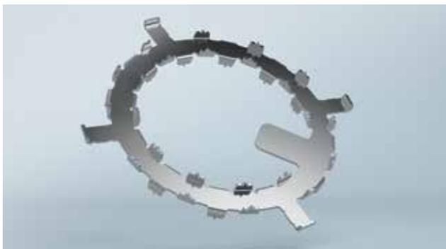
The great advantage of this solder-free design: it has completely excluded the risk of damaging the capacitor windings at the manufacturing stage due to overheating during soldering of the connecting leads. The quality of the winding connection is significantly increased, and the reliability of the mechanical fuse that protects against excessive internal pressure is improved by its being securely spot-welded in place.
