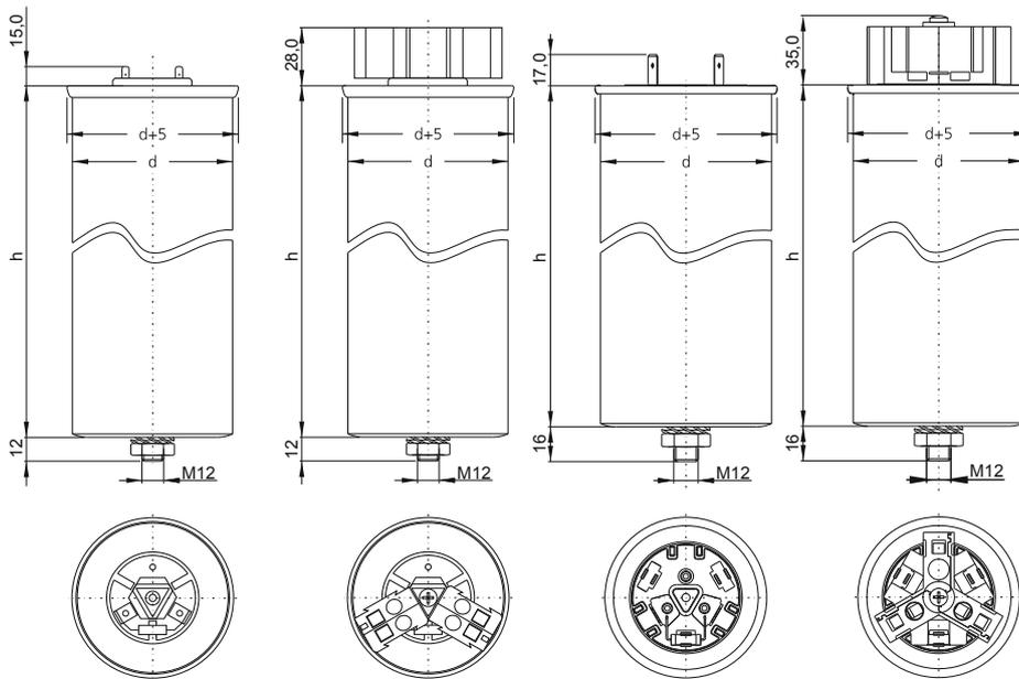
**Single-phase capacitor with d = 60/70 mm**
