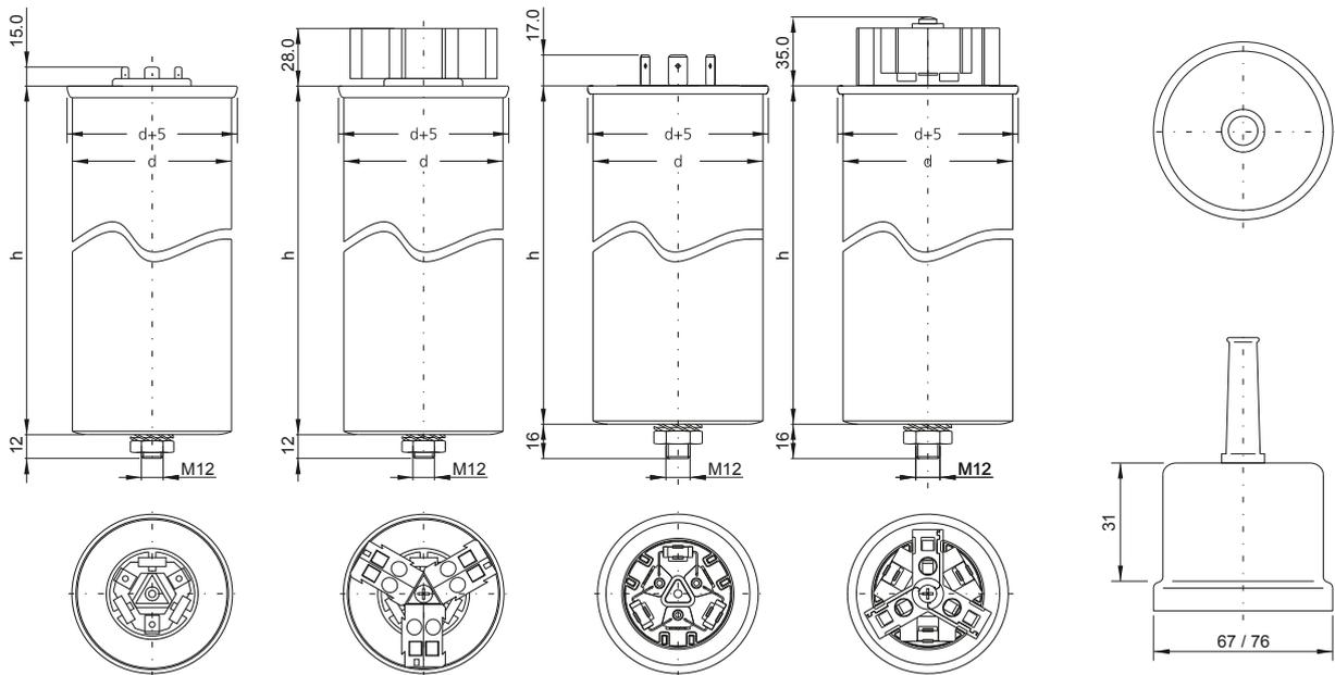
**Three-phase capacitor with d = 60/70 mm**
