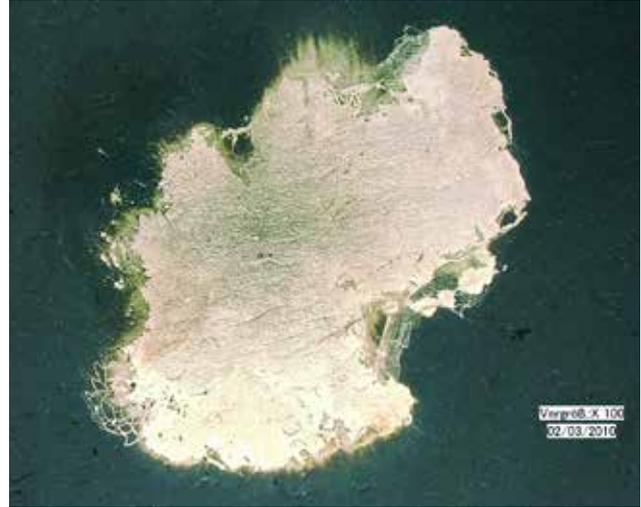
If several punctures occur in a small area of metallized film, the amount of energy involved might be too much for the **self-healing** action alone to cope with. This could lead to complete failure of the capacitor. However, in this case the second fail-safe function of the fourfold safety design comes into play: the **segmented metallization**.
